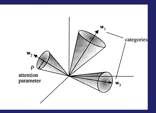
Illustration of the categories (or clusters) in input space formed by ART networks. Notice that increasing  $\rho$  leads to narrower cones and not to wider ones as suggested by the figure.
